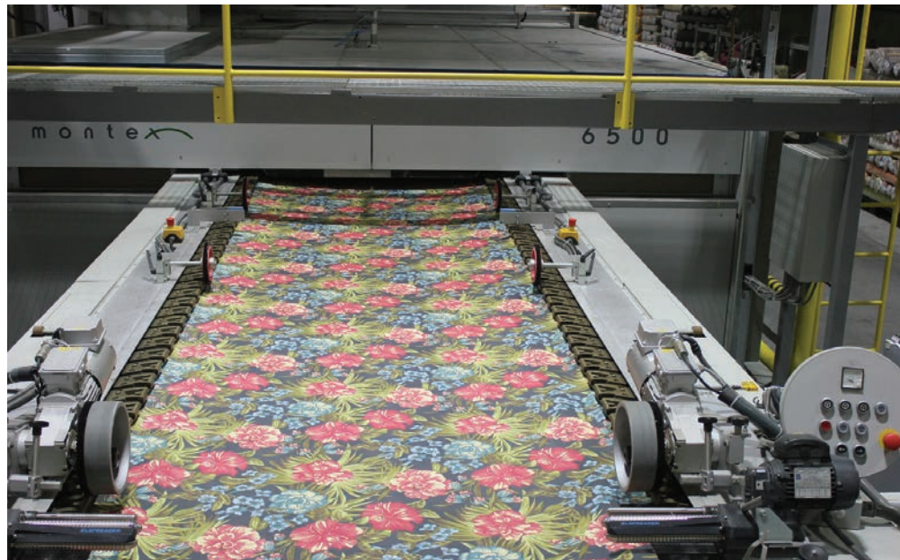
A new Monforts Montex stenter at Döhler in Santa Catarina, Brazil. The country's textile and apparel sector is the nation's second largest employer and $8bn has been invested in a recent upgradation project
